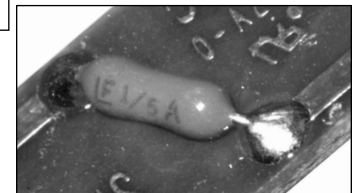
OEM Fuse Type 2 (Surface mount, insulated with leads) found in the drum unit
